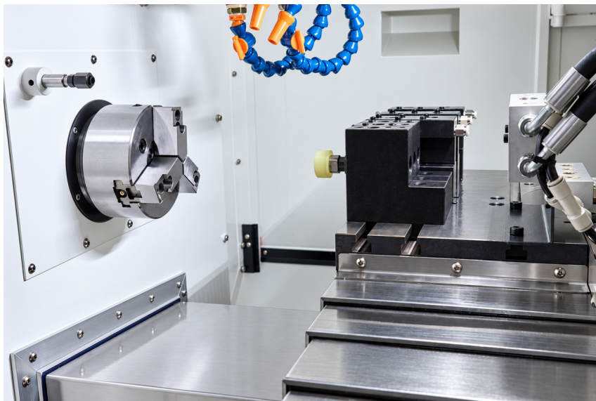
Spindle, workholding area and in-machine automation
